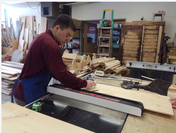
Owen Hughes uses the table saw to shape a plank for a steam box. Owen’s Senior Project revolves around the design and construction of a series of glued-up veneer longboard skateboards using several different construction methods, including steam bending and cold glue vacuum-bagging. Both the steam box and vacuum apparatus will subsequently be available as tools for other WLC students and classes.
