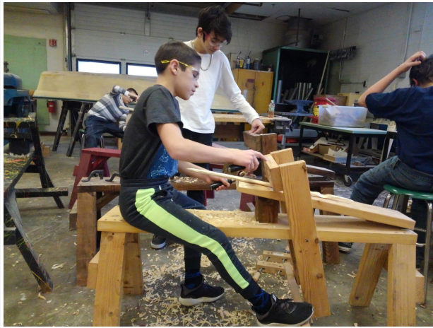
Ruben Sistachs and Rafael Maciel work on their carved wooden spoons in 8th grade Tech Ed. Ruben is using a 19th century drawknife and sitting at a shave horse, a medieval European woodworkers bench re-designed and built by a high school Woodworking class earlier in the year.
